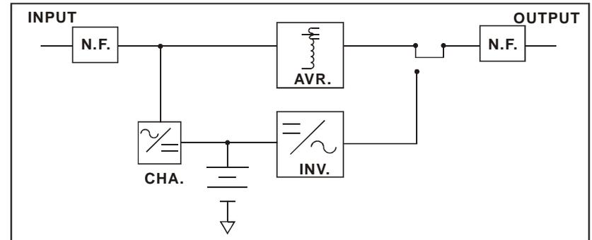
Fig. 1 shows how UPS works.
