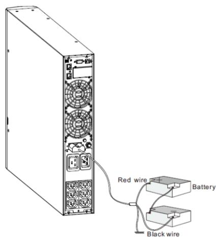
Figure 14 Long backup external battery connection
